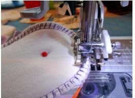
This time we are sewing around the outer edge of the pad body to attach the body top and bottom. Again, left hand stitch catching your fabric, right hand dropping just over the edge.
