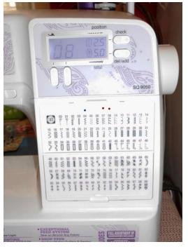
We're going to sew the pad core together first. You'll want to use an overcast stitch. On my machine, these are stitches 7 & 8. If you don't have an overcast stitch on your machine, a zig zag with a short length and wider width will work just fine.
