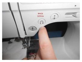
Place your pinned pad core pieces under the presser foot. You want your fabric right up to the edge so that the left hand stitch catches the fabric and the right hand stitch drops just over the fabric. Back-stitch (or reinforce) and then sew all along the edge.
