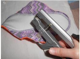
Press with your snap pliers or press using the manufacturers specifications for attaching a snap.
