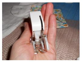
If your core is made up of stretchy fabric(s), use a walking foot. Follow your machine's instructions for installing it.
